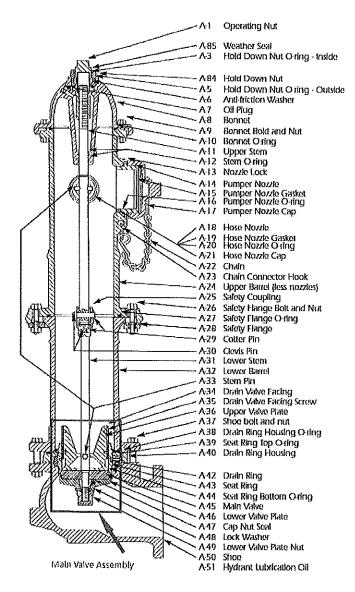
The Main Valve Assembly MVA is designed to be threaded out to be repaired or replaced with out excavation or replacement of the entire fire hyrant.
